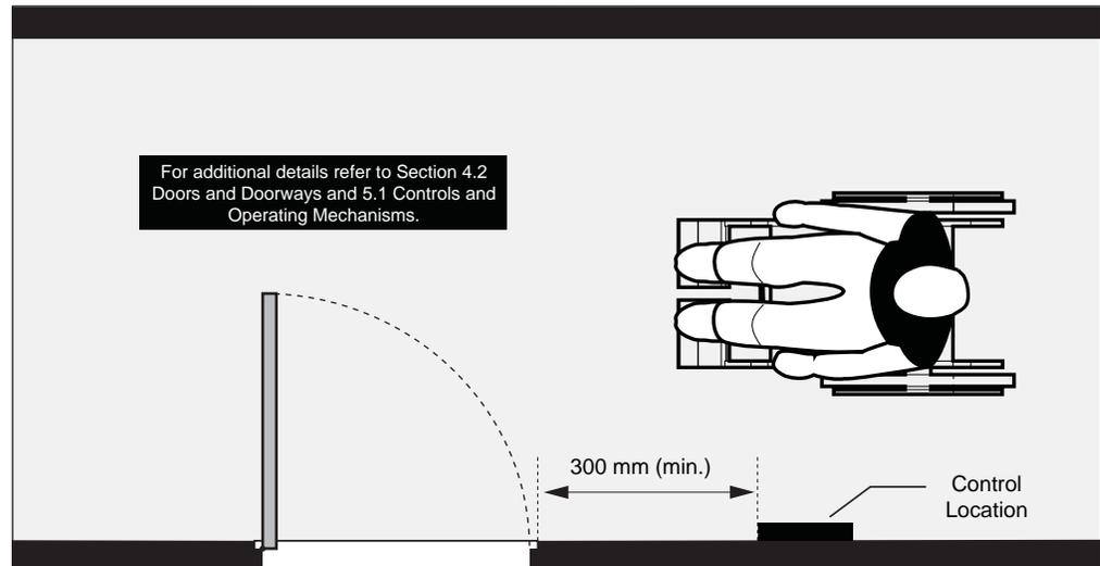
**Figure 67:** Proximity Card Reader Location - Plan View
