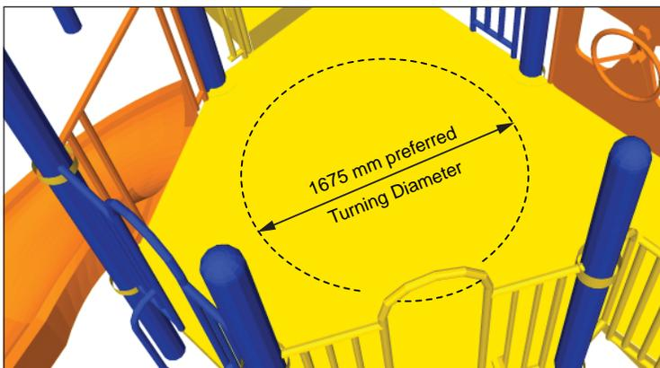
Figure 101: Turning Space - Plan View
