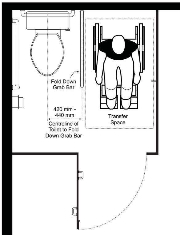
**Figure 56a:** Fold Down Grab Bars - Plan View
