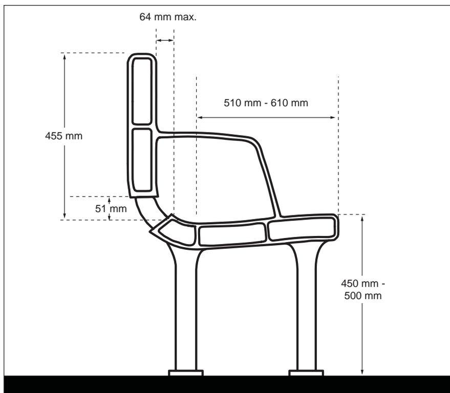
**Figure 22:** Typical Accessible Bench Dimensions - Section View
