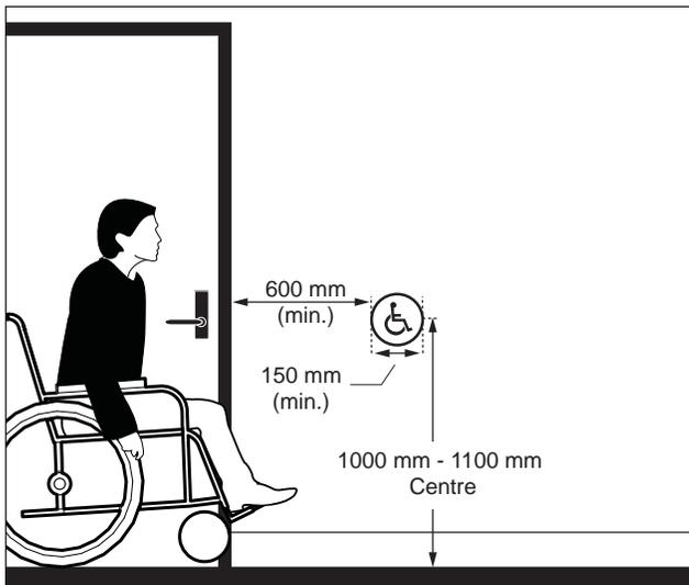
**Figure 40a:** Circular Push Button - Elevation View
