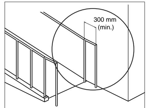
**Figure 7c:** Handrail Returns to Floor
