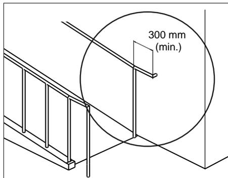
**Figure 7b:** Handrail Returns to Wall
