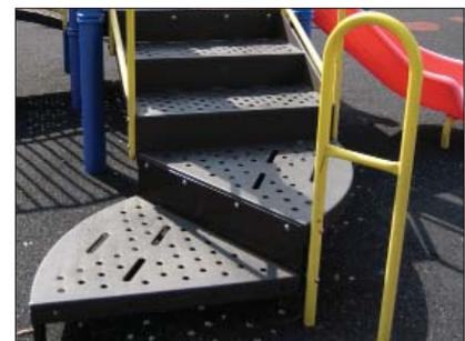
*Transfer system to connect elevated play components.*
