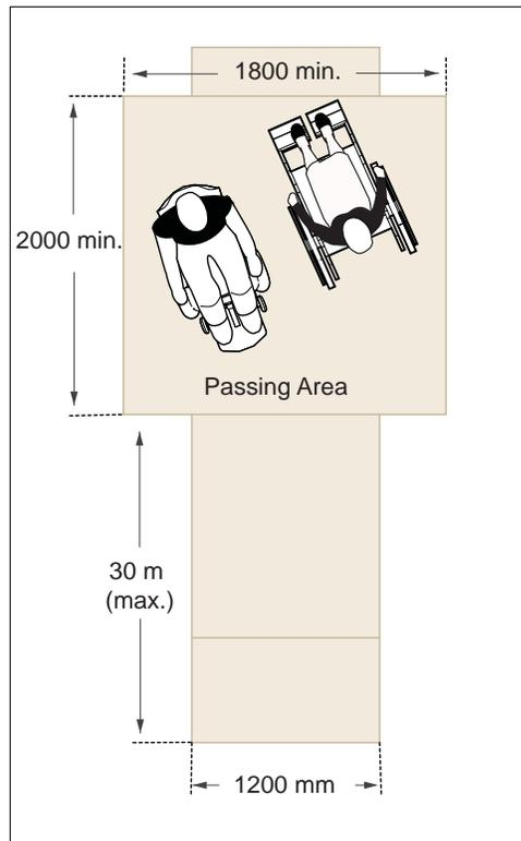
**Figure 29b:** Reduced Clear Width and Required Passing Area
