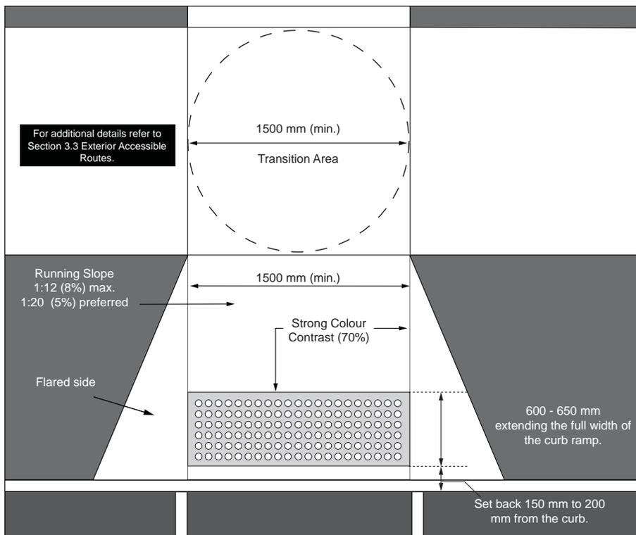
Figure 32: Typical Curb Ramp Design - Plan View
