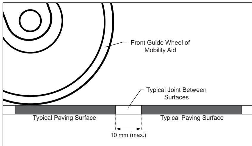
**Figure 1:** Joints Between Surfaces - Section View
