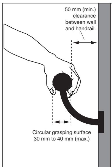
**Figure 13a:** Handrails on Wall - Section View
