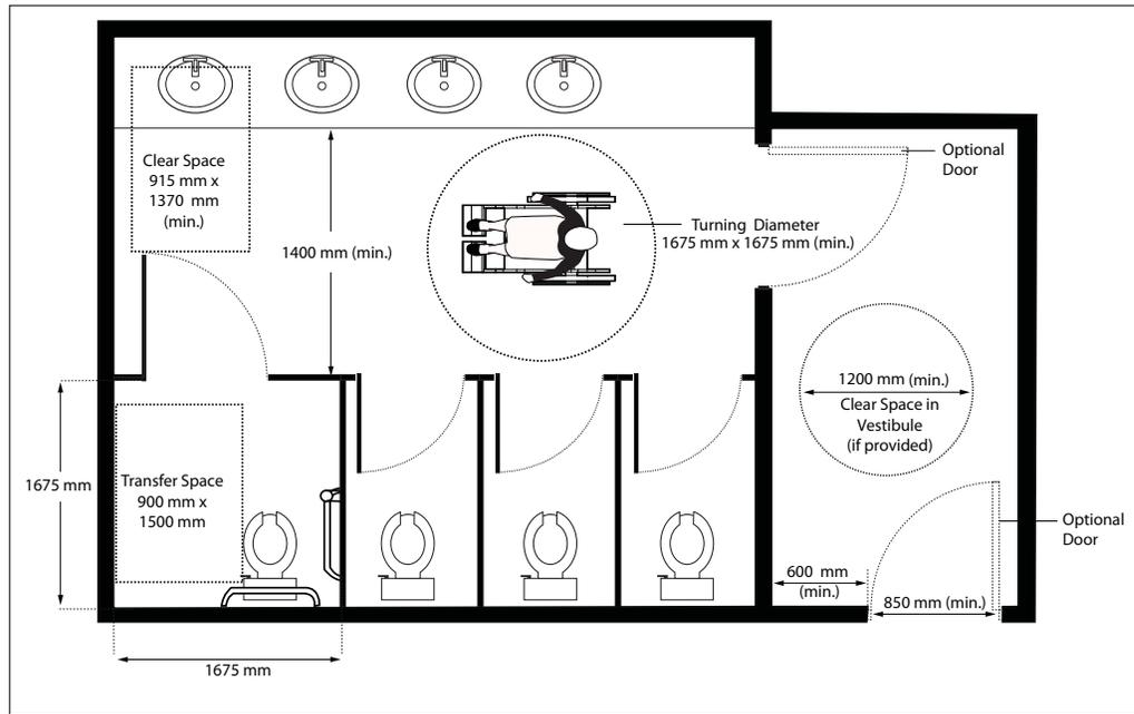
**Figure 50:** Example of Multiple Occupancy Washroom Layout
