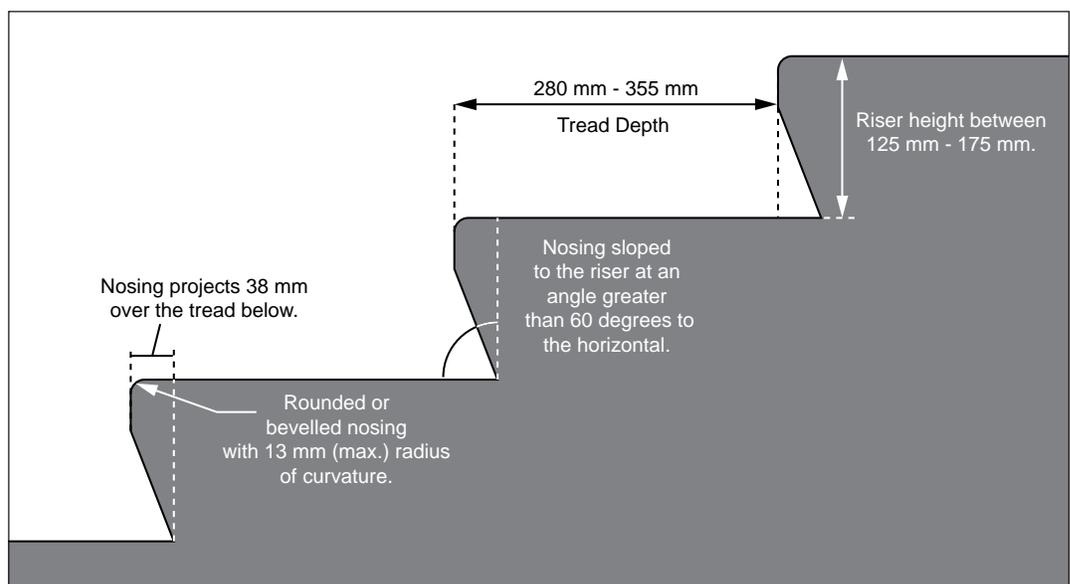
**Figure 10:** Stair Design Features - Section View
