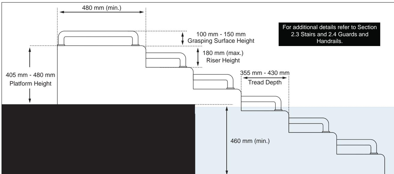
**Figure 89:** Transfer Stairs or Steps - Elevation View
