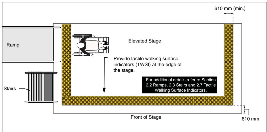
**Figure 95:** Elevated Platform or Stage - Plan View
