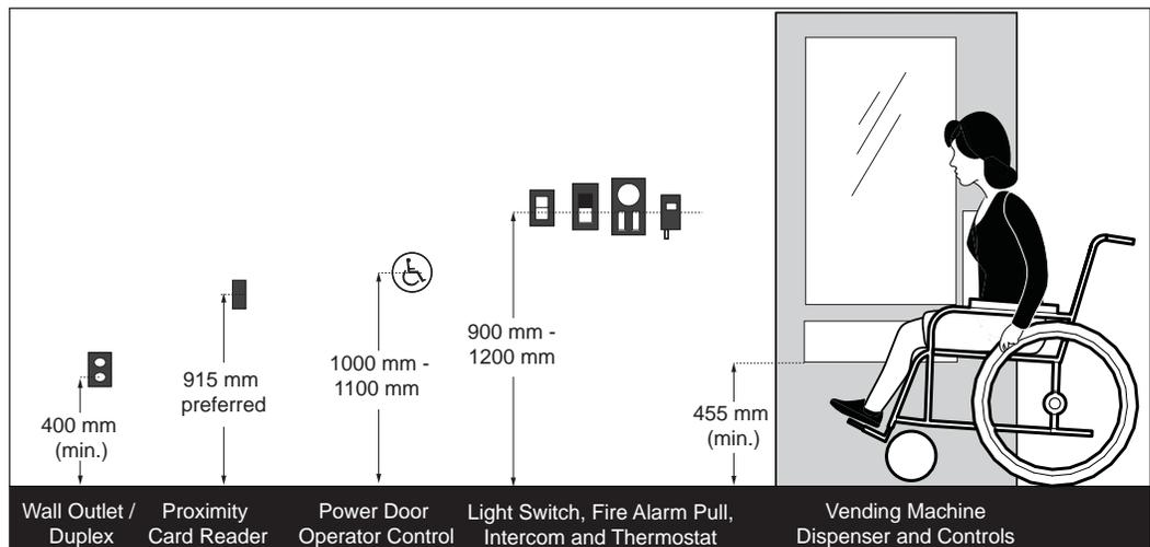
**Figure 64:** Control Mounting Heights - Elevation View
