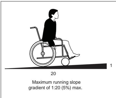
Figure 48: Running Slope
