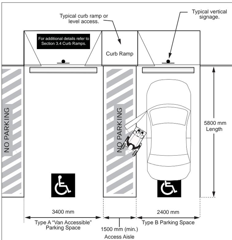
**Figure 24:** Accessible Parking Space Dimensions - Plan View
