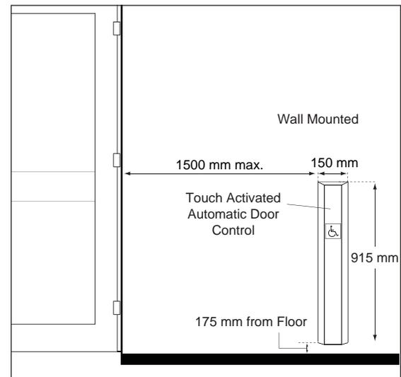
**Figure 40b:** Touch Activation Device - Elevation View
