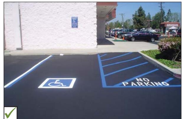
*Locate accessible parking space as close as possible to accessible entrance, with accessible route integrated.*
