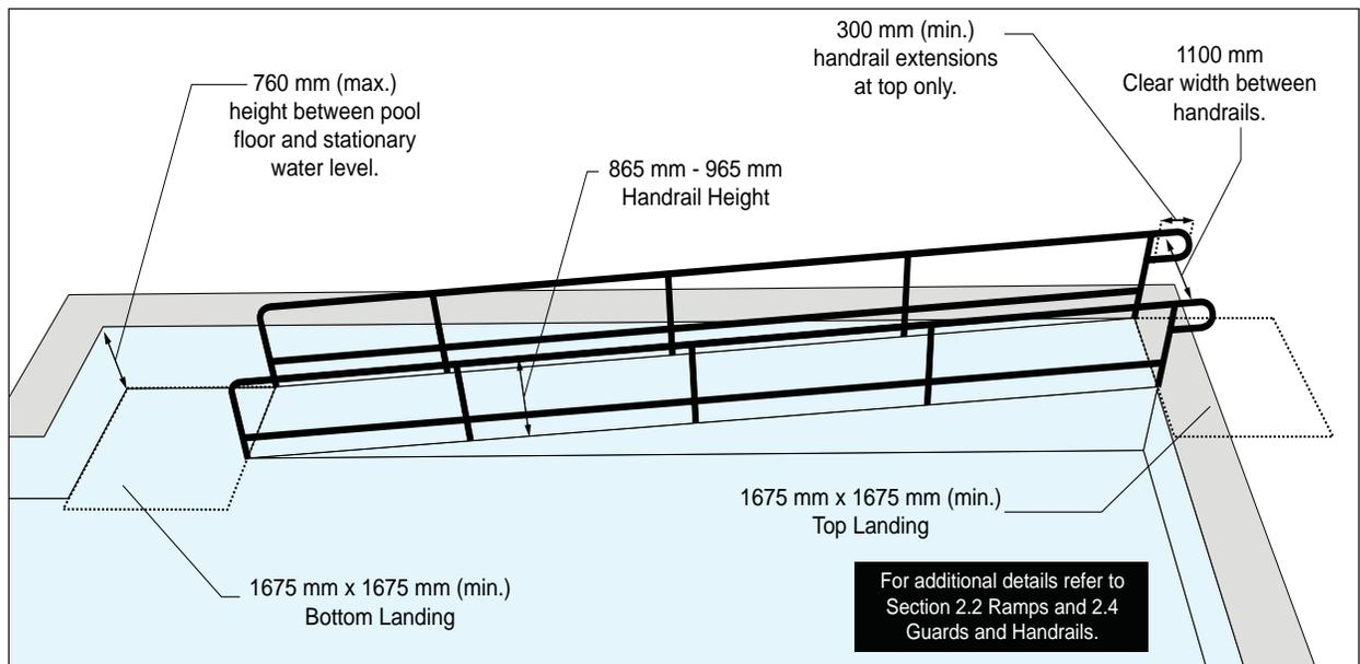
**Figure 88:** Sloped Entry or Ramp to Swimming Pool
