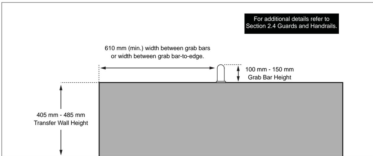
**Figure 90:** Transfer Wall - Elevation View
