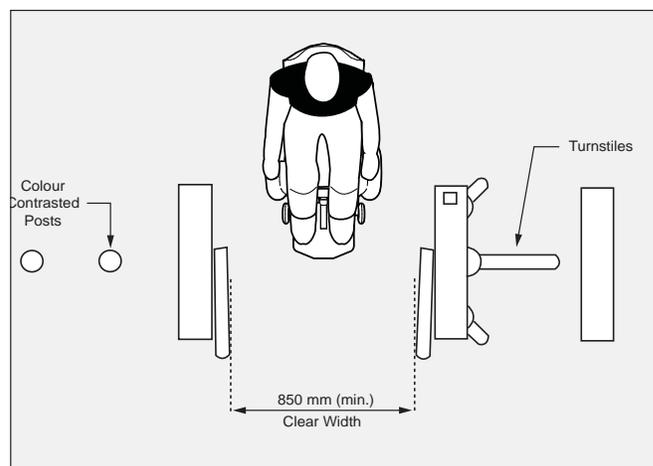
**Figure 38:** Accessible Controlled Gate
