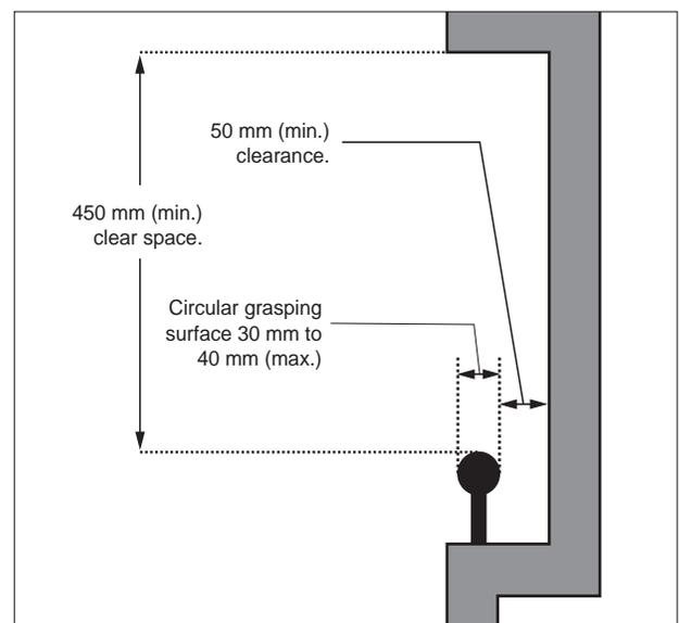
**Figure 13b:** Handrails in Recessed Area - Section View
