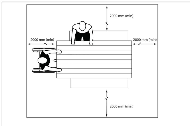
**Figure 96a:** Picnic Table Design and Features - Plan View
